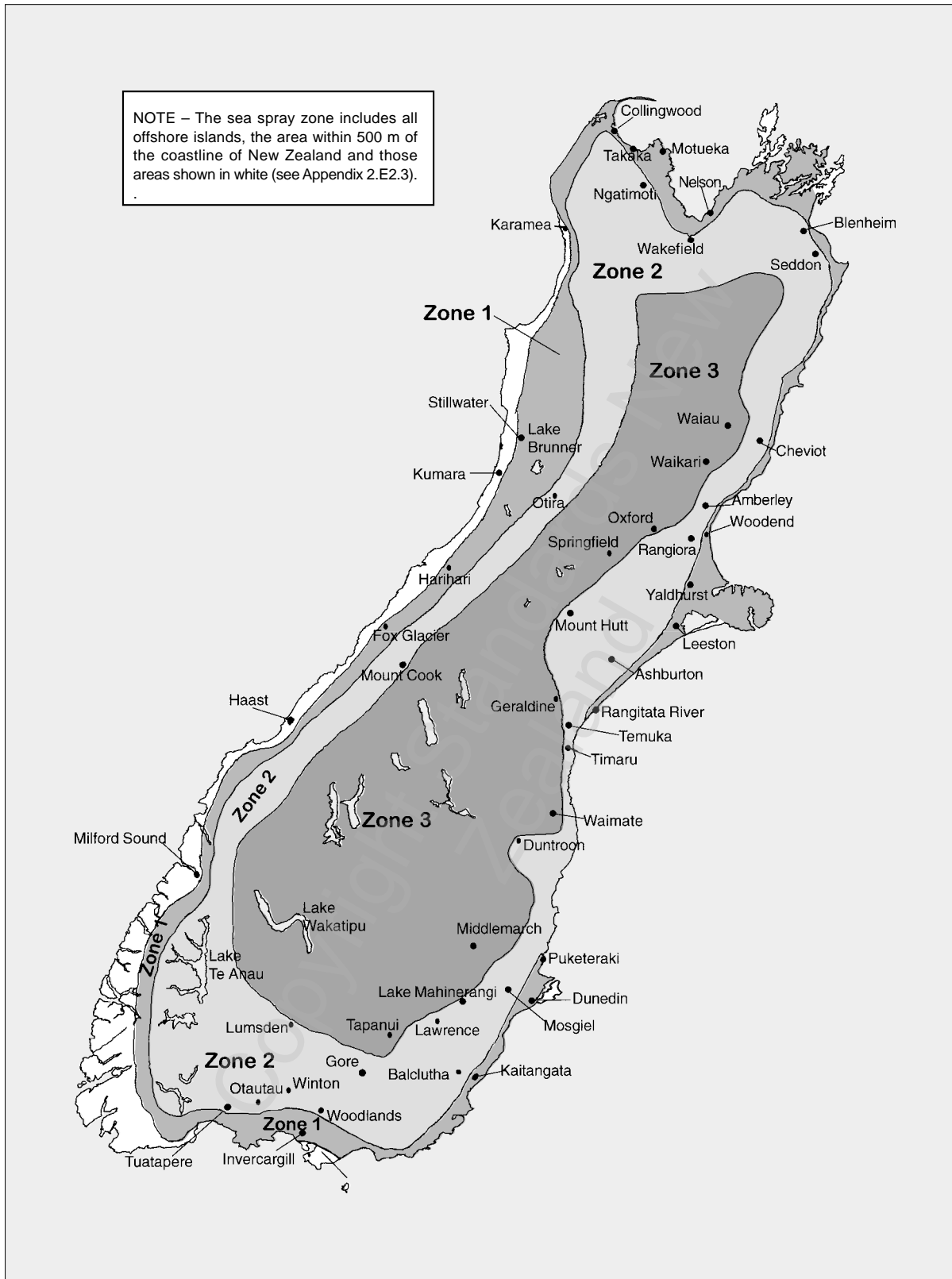
Figure 2.E1 – Corrosion zone map (continued)
